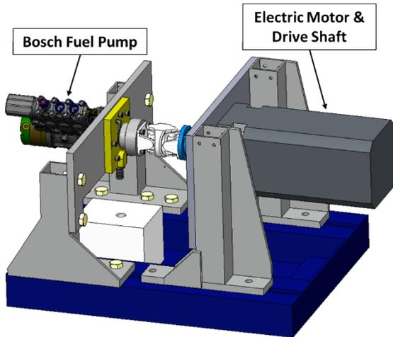
Figure 4 – EFI Pump Test Rig Concept
