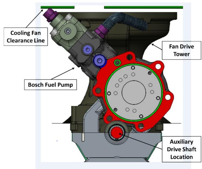
Figure 3 – EFI Pump Mount Orientation
