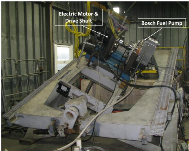
Figure 5 – EFI Pump Tilt Test
